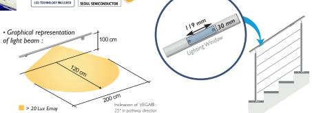
Graphical view of mounting showed inside the handrail tube :
